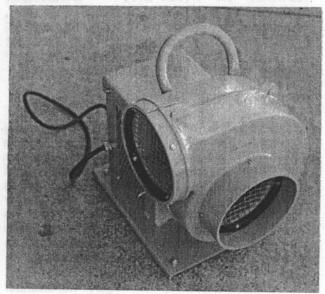
5) Do not operate the Blower without the inlet and outlet screens properly secured and in place. Never replace the screens with other than factory supplied, replacement units. The screen grid must comply with current OSHA regulations regarding protective enclosures to prevent personal injury to the operator(s). Determine that the structural integrity of the screens will allow them to serve their protective function. Keep both screens free
