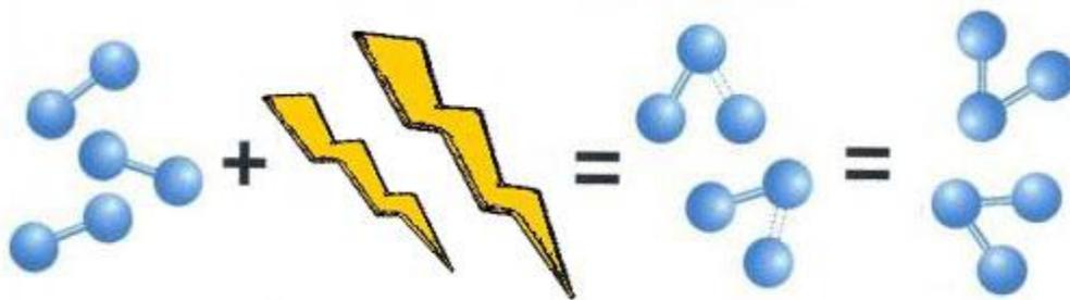
3 Oxygen (O<sub>2</sub>) + High Voltage = 2 Oxygen (O<sub>2</sub>) + oxygen (O) + oxygen (O) = 2 Ozone (O<sub>3</sub>)
