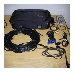
Position projection system 18-20 feet away from movie screen. Reverse image if using rear projection. Press "menu" button on projector remote. Select "management". Arrow down to "projection". Arrow over until image reversed. Select enter and then exit menu.
